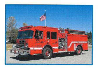
Figure IX-15: Engine 2 – 2008 Spartan/Smeal Pumper 1250 GPM pump capacity – 1500 gallon water tank Very good condition
