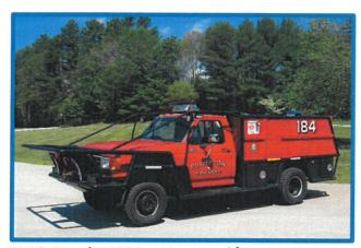
Figure IX-19: Breaker 184 – 1991 Ford/EJ Murphy Brush Truck 200 GPM pump capacity – 450-gallon water tank Fair condition
