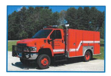
Figure IX-16: Engine 3 – 2007 GMC Danko pumper 110 GPM pump capacity – 400-gallon water tank 10-gallon foam tank Good condition.
