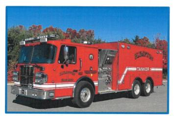
Figure IX-17: Tanker 1 – 2013 Spartan/EVR pumper tanker 1500 GPM pump capacity – 3000-gallon water tank Excellent condition
