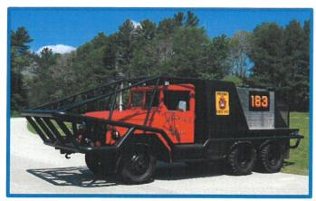
Figure IX-18: Breaker 183 – 1974 AM General Brush Truck 250 GPM pump capacity – 750-gallon water tank Fair condition.
